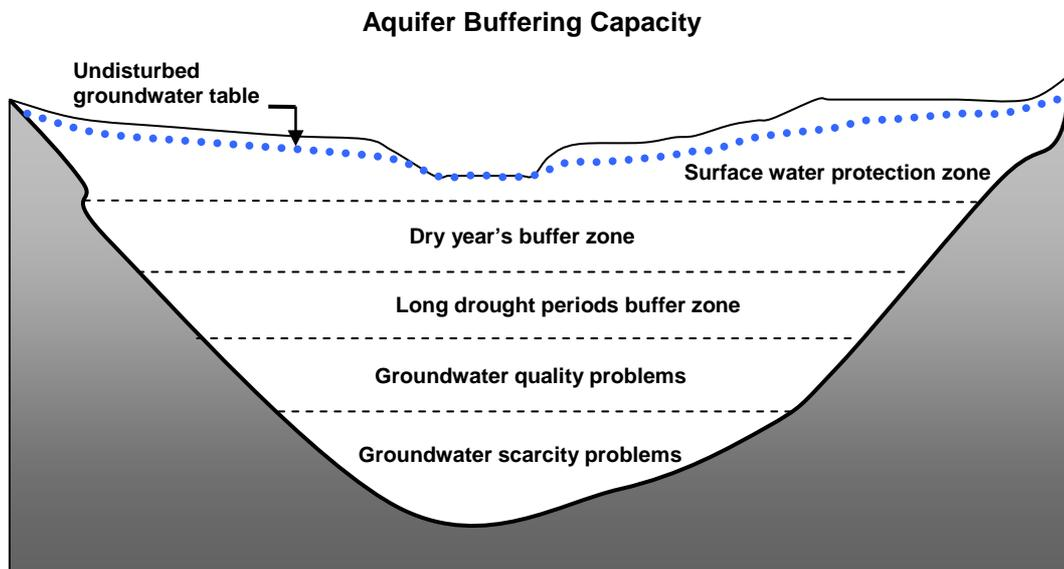
**Figure 7: Buffer zones for a groundwater aquifer.**
