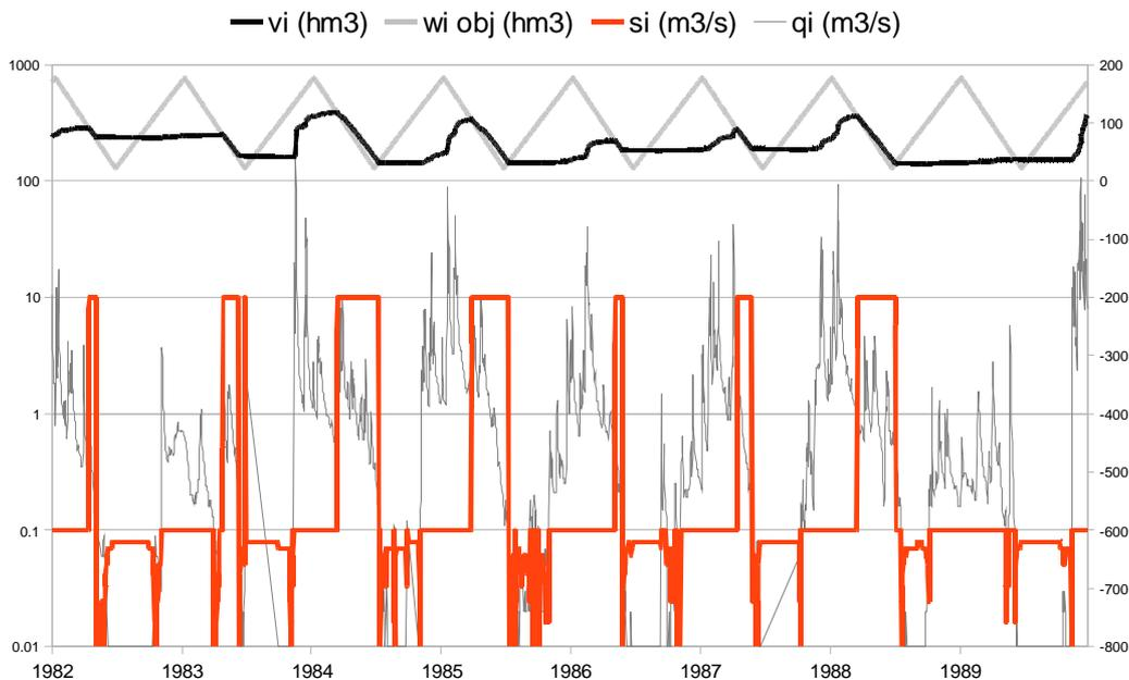
**Figure 6: Observed upstream flow ( $q_i$ ), calculated downstream flow ( $s_i$ ), target volume ( $w_i$ ) and calculated stored volume ( $v_i$ )**
