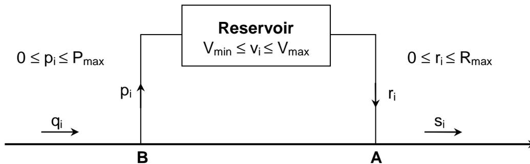
Figure 2: Functioning of a reservoir used for flow regulation
