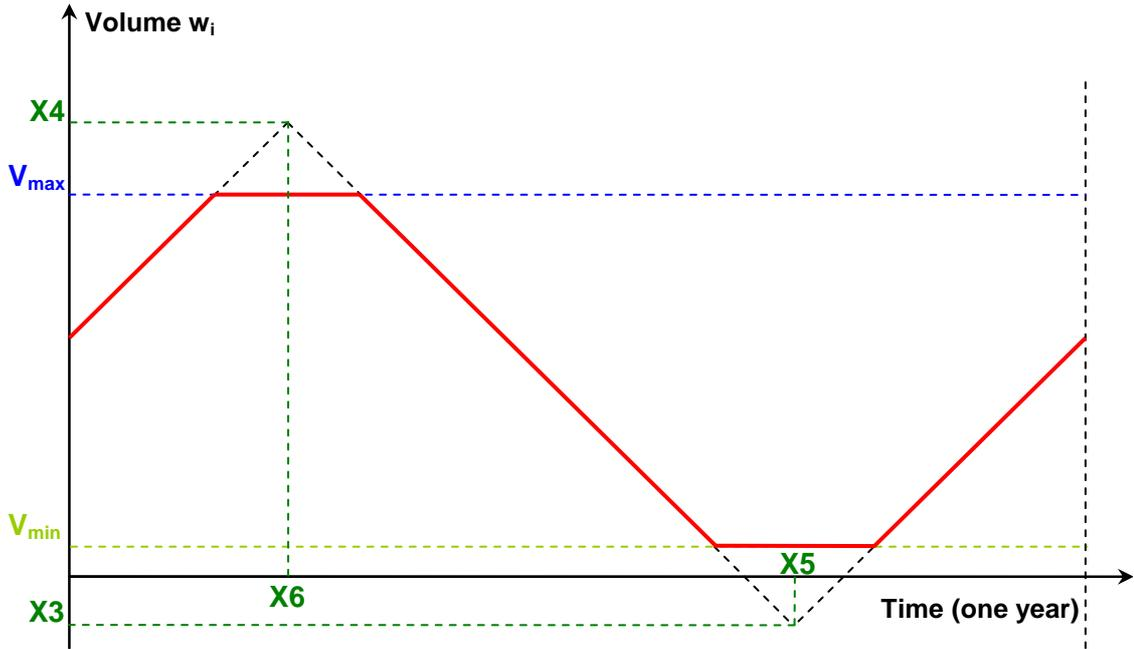
**Figure 4: Parameterised annual plan of operation for a reservoir**
