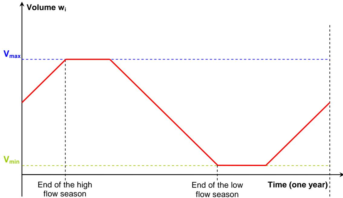
**Figure 1: Example of a basic annual plan of operation for a reservoir**
