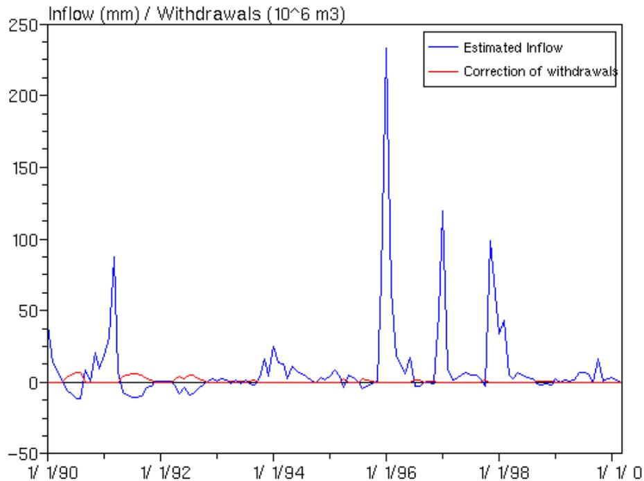
**Figure 7:** Estimation of Caia reservoir inflows based on stored volumes and water withdrawals data
