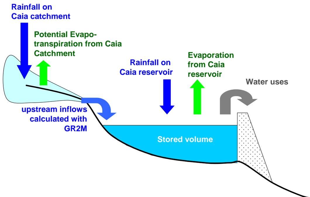
**Figure 4:** Model structure used to simulate monthly stored volumes in the Caia reservoir
