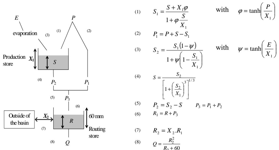
**Figure 5:** Sketch of the GR2M model (E: potential evapotranspiration; P: rainfall; Q: streamflow; X1 and X2: model parameters; the other letters are model internal state variables)
