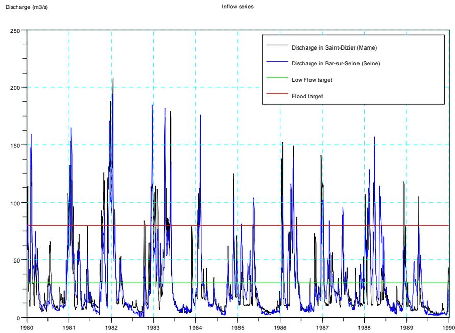
**Figure 10:** Reservoirs inflows (m<sup>3</sup>/s) with low flow and flood regulation objectives
