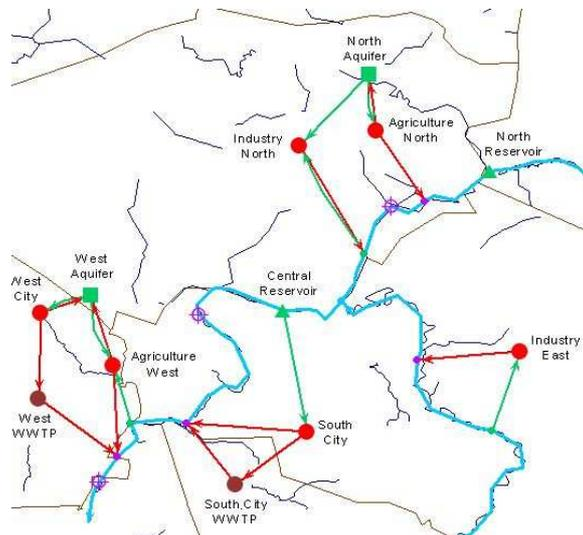
**Figure 18** : Network representation of hydrosystem (WEAP software)
