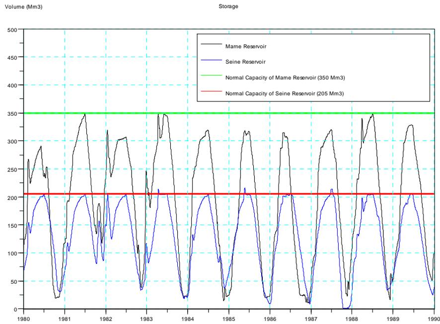
Figure 12: Reservoirs storage with normal capacity (Mm3)
