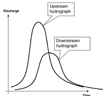
**Figure 2:** Buffered hydrograph
