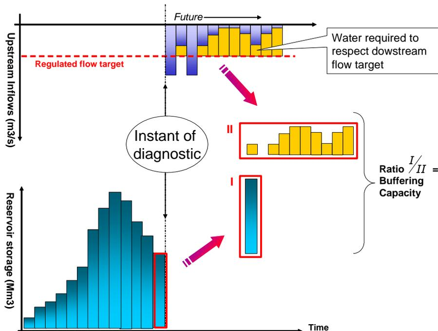
**Figure 9:** Storage capacity and respect of downstream flow targets
