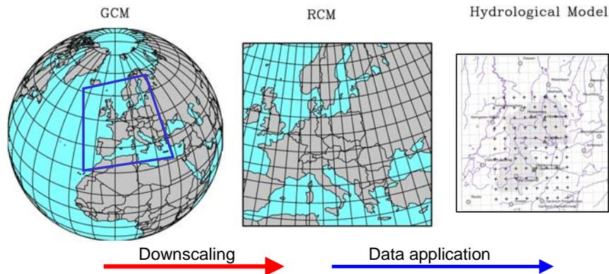
**Fig. 1** Principle of downscaling of global climate change data.
