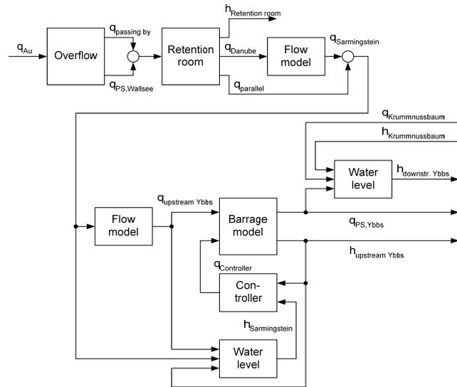
Fig. 4 Simulation model structure for reservoir Ybbs
