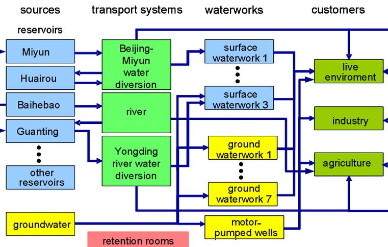
Fig. 2 Structure of the Beijing water supply system
