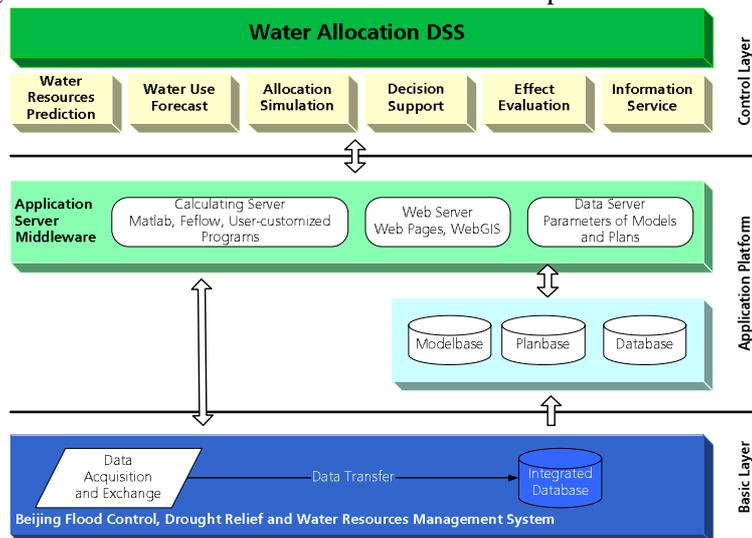
Fig. 1 The logical structure of the "Capital Water Resources Allocation Decision Supporting System"
